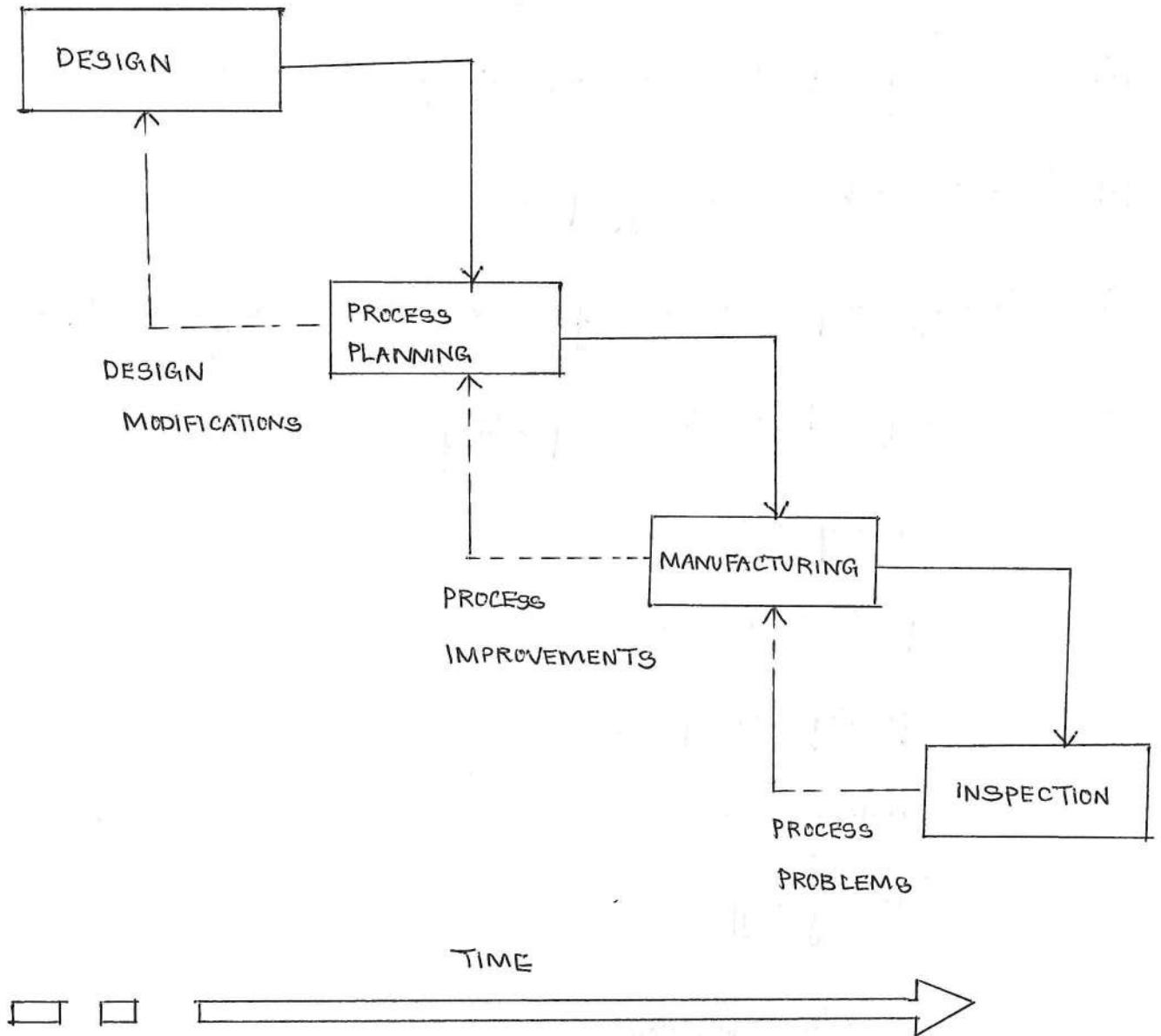
The design and manufacturing time i.e., the time to market has to be shortened as much as possible by the system. For that purpose, cross-functional teams are employed to simultaneously work on the design and manufacturing functions. This approach is known as simultaneous or concurrent engineering.
